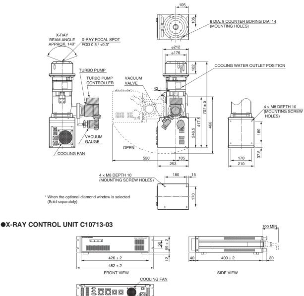
System configuration of L10713-03: X-ray tube unit (L10712-03) + X-ray control unit (C10713-03) + turbo pump set + accessories
