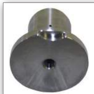
Bottom of reflection target indicating beam direction
